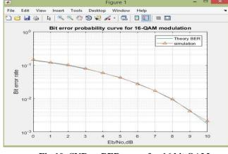
Fig 10: SNR vs BER curve for 16 bit QAM
