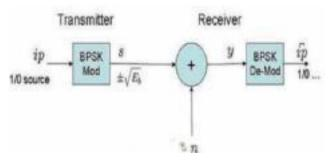
Fig 2: BPSK Transmitter and Receiver
