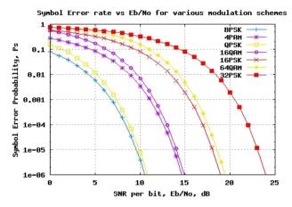
Fig 11: Theortical SNR vs BER curves for various Modulation Schemes
